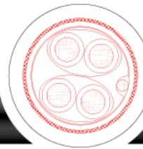
Instrumentationcable +90°C / 300 V
