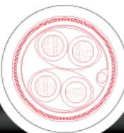
Instrumentationcable +90°C / 300 V
