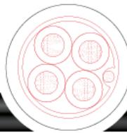
Instrumentationcable +90°C / 300 V
